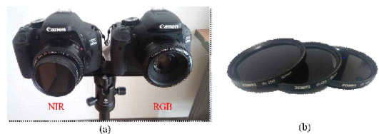
Fig. 1. (a) The Camera for NIR and RGB image (b) NIR filter(720nm, 850nm, 950nm)
