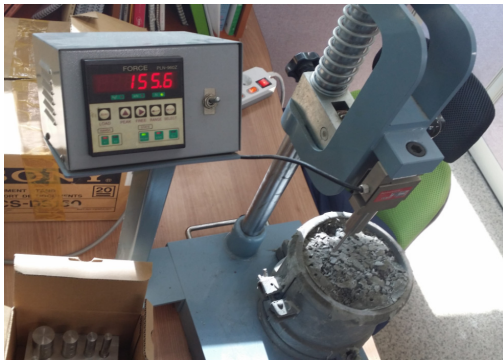
Photo 3 Penetration resistance test
