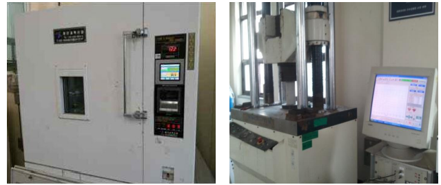
Photo 4 Isothermal-isohumidity chamber and 200 ton UTM
