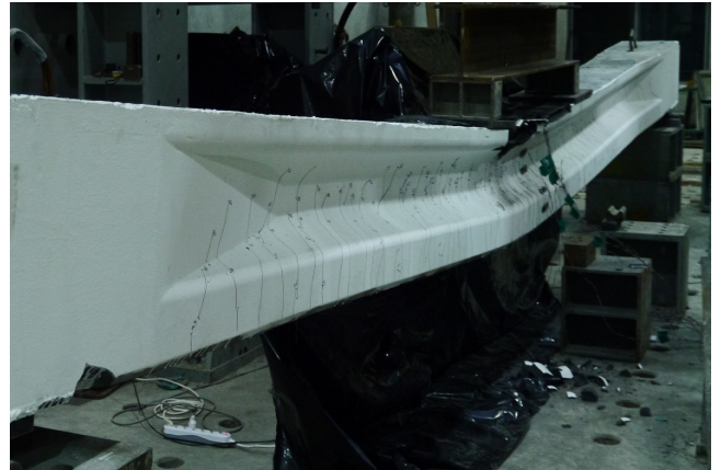
Photo 2 Deflection Patterns of F0S2 Beam
