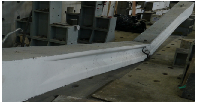
Photo 8 Deflection and Failure Patterns of F2 Beam
