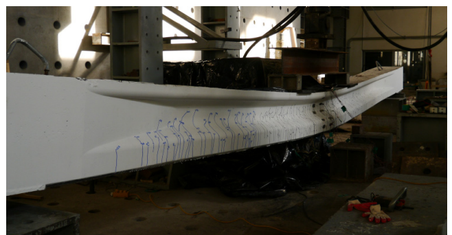
Photo 4 Deflection Patterns of F0.7S2 Beam
