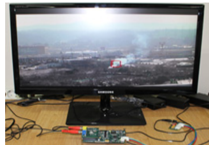
Fig 11. Test picture for smoke detection using DSP board of vision sensor
