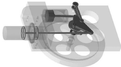
Fig. 14 Designed \gamma -type Ross yoke driver stirling engine
