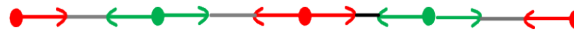
Fig. 7(a). When sensing radius is less than L/2 , sensing regions of all the sensors will not intersect with each other.
