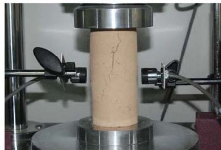
(b) A specimen after unconfined compression test
