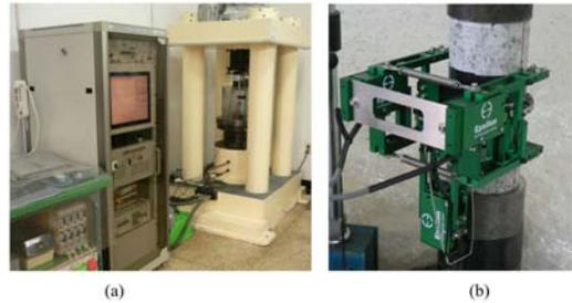
**Fig. 4.** Equipment used for damage-controlled tests: (a) stiff compression machine; (b) devices for measuring displacement.
