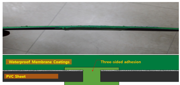
Fig. 7. Three-sided adhesion of joint
