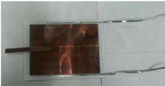
Fig. 1 Fabricated module and copper electrode
