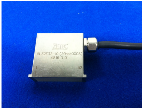
Fig. 5 Phased array transducer
