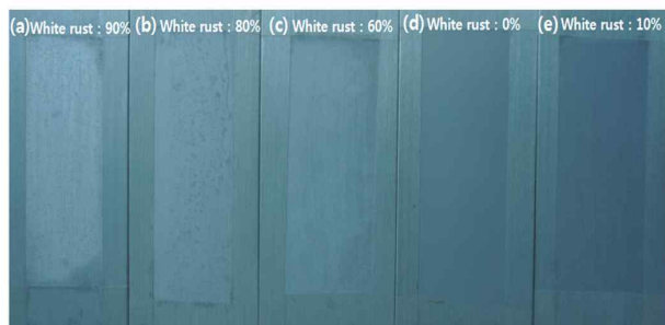
Fig. 7. Corrosion resistance for F-coating films containing various F-WPUs on electro-galvanized steel sheet: (a) F-Coating01, (b) F-Coating02, (c) F-Coating03, (d) F-Coating04, and (e) F-Coating05.
