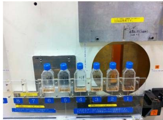
Fig. 1. Cell irradiation in HIMAC (Heavy Ion Medical Accelerator in Chiba).
