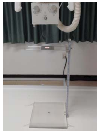
Fig. 1. The experimental setup for half value layer measurement.
