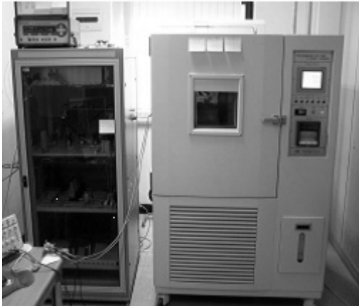
Fig. 2 Experimental apparatus: constant temperature and humidity chamber (right side), MFC controller (left side), a multi-gas analyzer above MFC (left top side).
