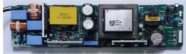
(a) LED PSU board with the individual inductor and transformer
