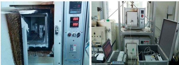
Figure 1. Thermocouple position and calibration test
