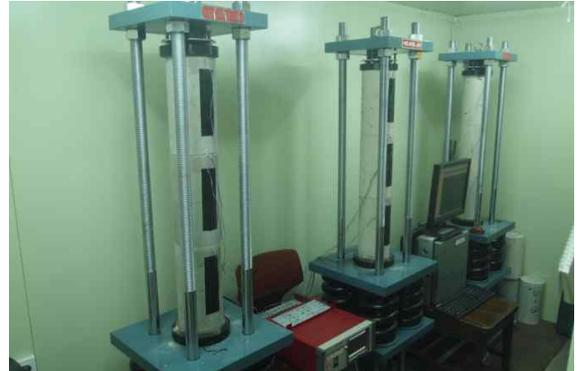
Figure 1. Creep test
