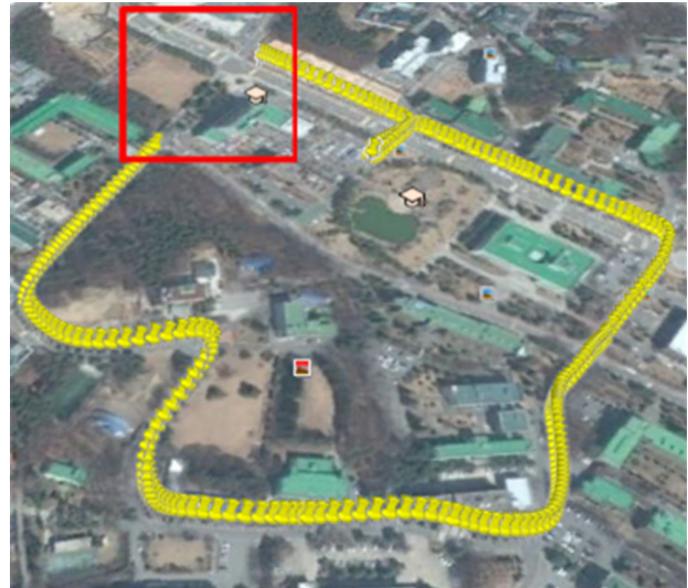
Fig. 9. Area where GNSS signals are not available in the driving path.
