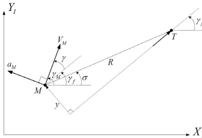
FIGURE 1. The planar homing engagement geometry
