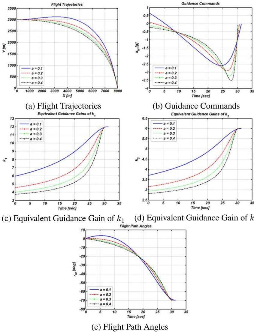
FIGURE 3. Simulation results of proposed impact angle control laws for various design parameters
