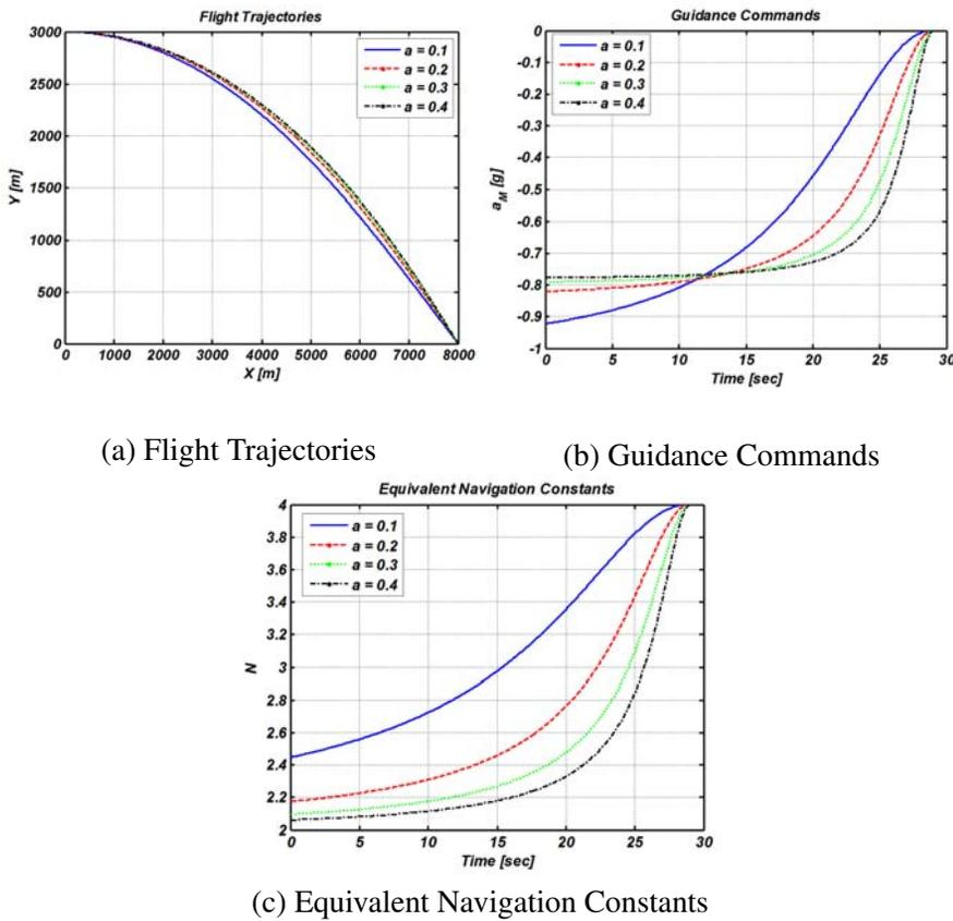
FIGURE 2. Simulation results of proposed homing guidance laws for various design parameters
