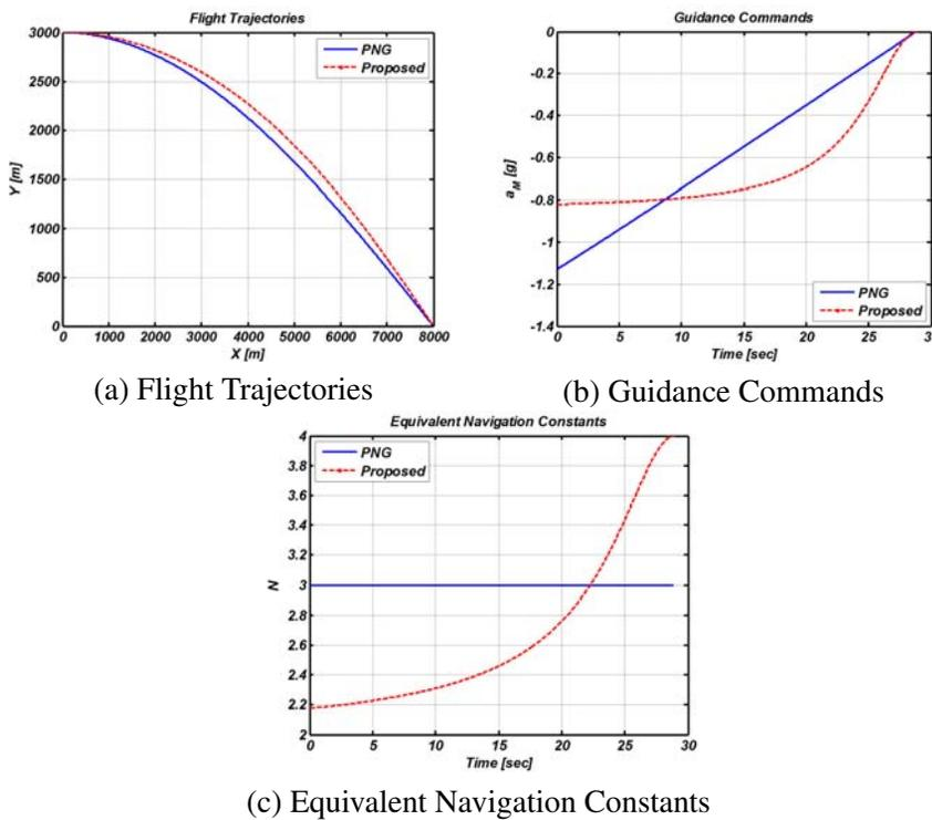
FIGURE 4. Simulation results under PNG and the proposed guidance law in the case of interception
