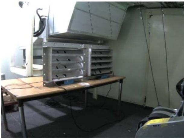
Fig. 6 Photography of the ice class louver installed heating cable in the cold-chamber
