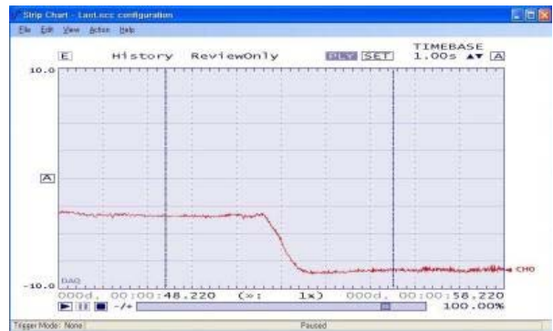
Fig. 4 LVDT voltage output corresponding to ice sheet deflection
