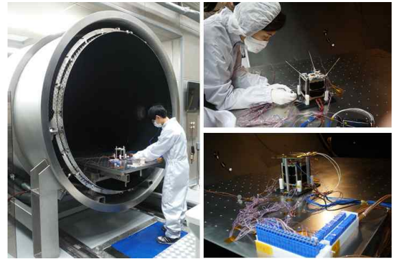
Fig. 9. FM T/V Test Set-up Configuration
