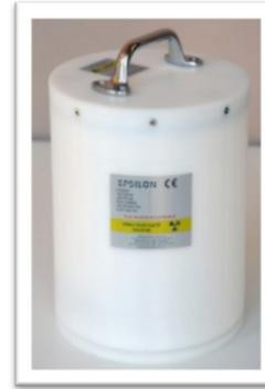
**Fig. 3.** <sup>68</sup>Ge cylinder phantom was used for Daily PET QC at Siemens PET/CT scanner.
