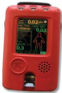
Fig. 9. PERSONAL ELECTRONIC DOSEMETER(PED) was used to measure occupational radiation dose manufactured by Tracerco™.
