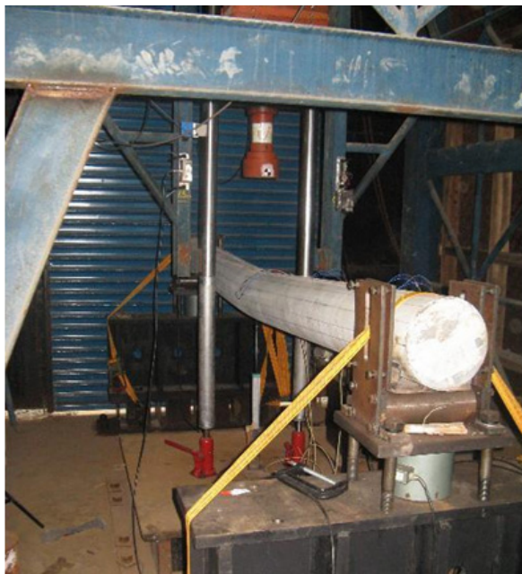
(a) Lateral impact of CFT columns
