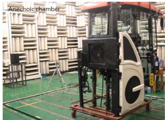
Figure 3. Cabin sound insulation test set.
