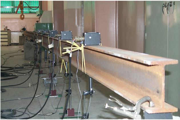
Photo 1 H-Beam Test Set-Up
