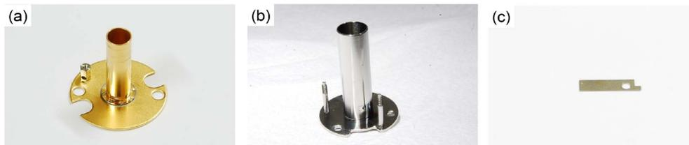
Fig. 3. Anode chamber of QMS after the cleaning (a) CPM-300, (b) Prisma 80, (c) Repeller of CPM-300.
