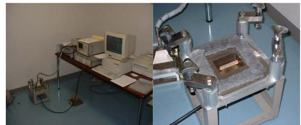
Fig. 7. Measurement system for electromagnetic interference shielding effectiveness (EMI SE) by KEC method.
