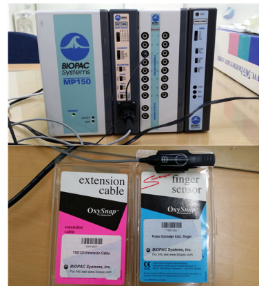
Fig. 6. BIOPAC MP150 with PPG module(BIOPAC Systems, Inc).
