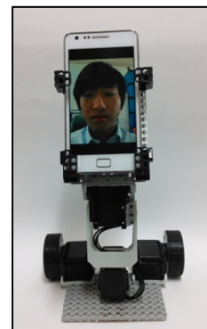
Fig. 5. A cost-effective implementation of the remote-side robot system.
