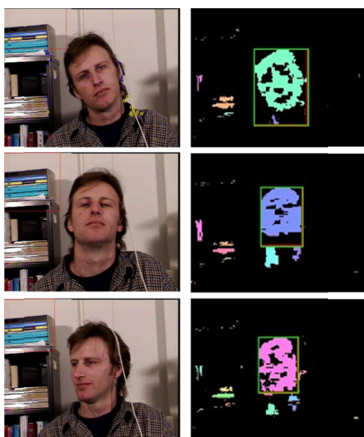
Fig. 6. Comparative results of face detection experiments: (Left) Failure of Viola-Jones method, (Right) Success of the proposed method
