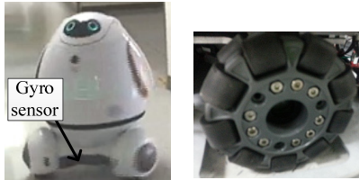
Fig. 5. Omni-wheel platform and its wheel.
