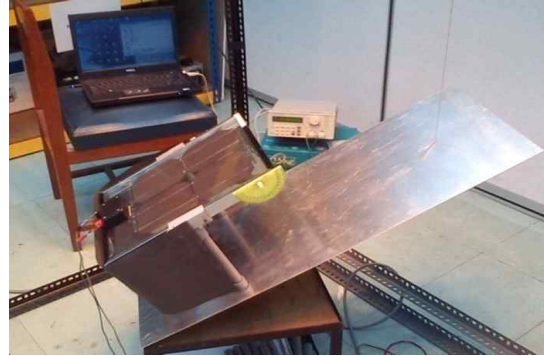
Fig. 1 Experimental configuration for indoor bifacial solar panel integrated with an external reflector.
