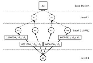
Fig. 5. Transmission of the split packets
