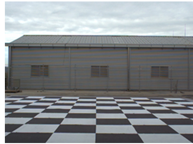
Fig. 1 Calibration pattern-based extrinsic parameter estimation needs a huge calibration pattern and wide flat plane
