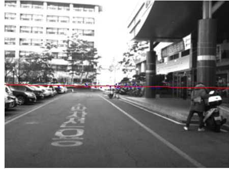
Fig. 6 Detected vanishing points and line of the second test set with small tilt and roll angle
