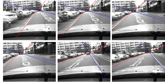
Fig. 3 Test images are captured while changing the horizontal angle with respect to lane markings. In each image, left and right lane marking is detected, and vanishing point is detected by finding their cross point
