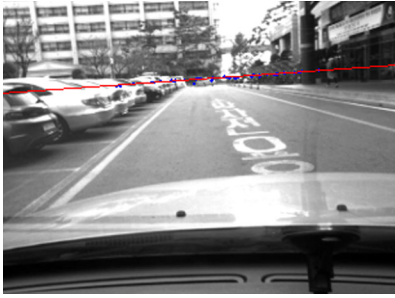
Fig. 4 Vanishing line is detected by fitting detected vanishing points (blue dot) into a line (red line)
