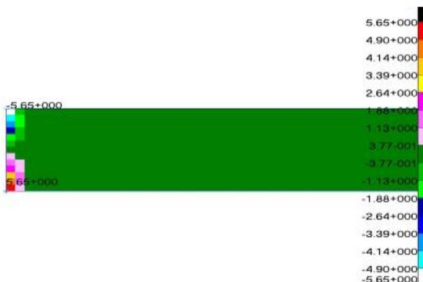
(c) Result of XY direction stress at the 0° top layer
