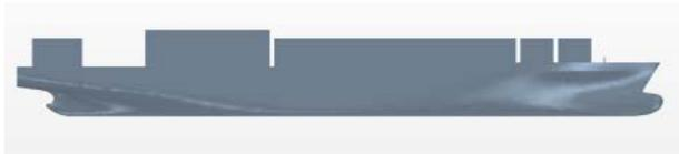
Fig. 1 Geometry modeling of KCS for CFD analysis
