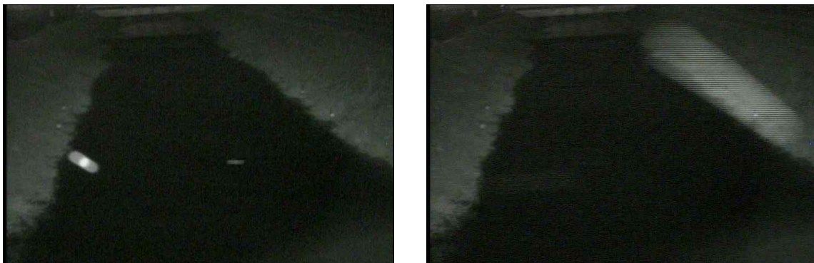
Fig. 5. Noise Images Due to Bugs or Flying Debris in Near Infrared Camera Images
