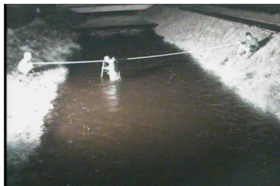
(b) Measurement using micro velocimeter
