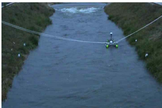
(a) Measurement using ADCP
