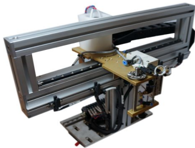
(a) Photograph of gear transfer mechanism
