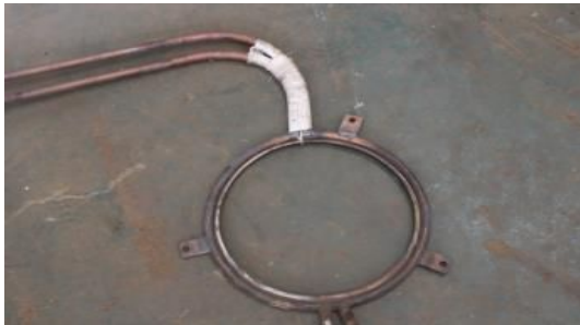
Fig. 5 Coil of asymmetry heating bending
