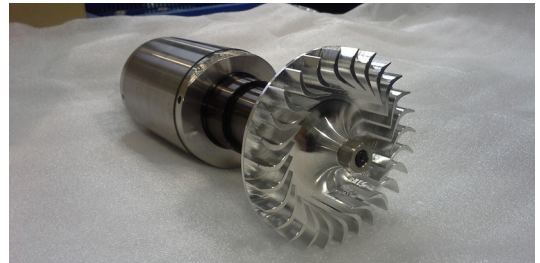
Fig. 4 Picture of turbine rotor connect with the generator rotor
