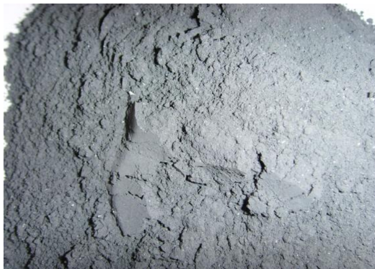
Figure 2. Aluminium dross that was crushed, sieved and classified to be not larger than that of the 200 mesh number.
