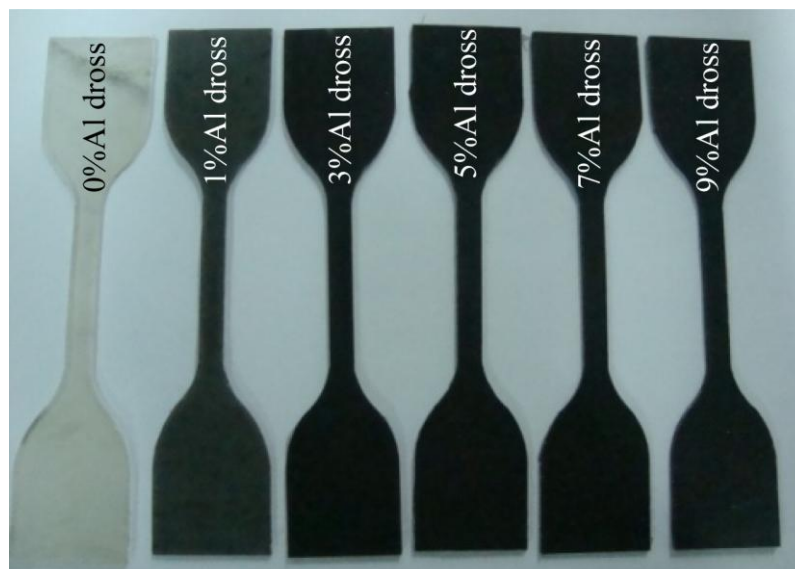
Figure 7. Tensile strength specimen follows ASTM D638 Type IV.
