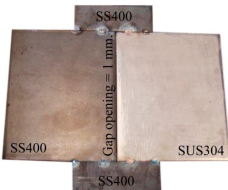
Figure 1. a set up of the butt joint.
