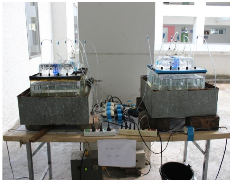
(b) A constructed immersion test chamber
