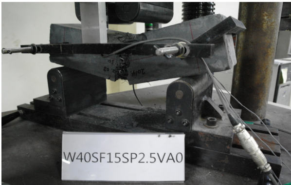
Fig. 10 High ductile behavior in bending test
