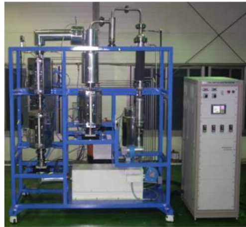
Fig. 1 Schematic of lab-scale CFB reactor to investigate the co-combustion with coal and wood pellet
