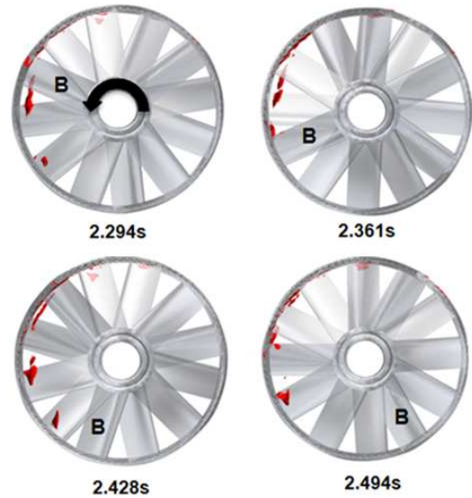
Fig. 9 Time dependent variation of cavitation generation region according to changes of the helical blade azimuthal angle
