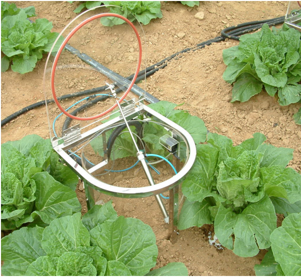
Fig. 1. Steady-state chamber for collecting N 2 O in soil.
