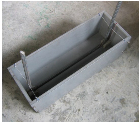
Fig. 7. Form to produce a concrete sample
