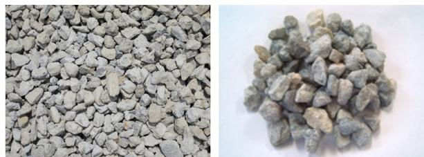
(a) Crushed stone (b) Recycled aggregate
